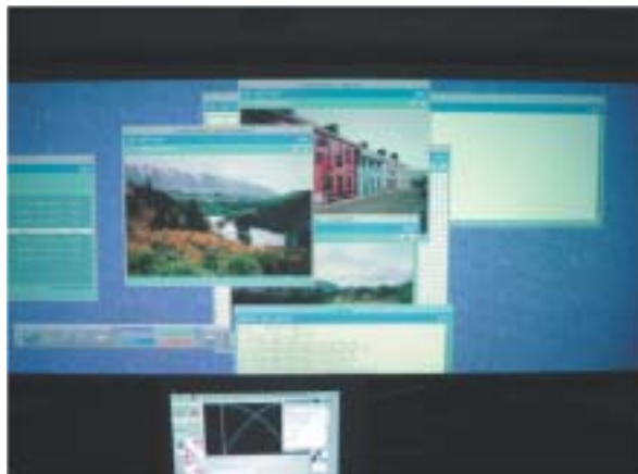
Dual Screen Edge Blended Rear Projection Display Showing Blendzone
