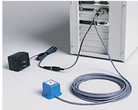
3D-BIRD sensor connects directly to the RS-232 serial port of your host computer. Sensor data is processed by the 3D-BIRD driver residing in your computer.
